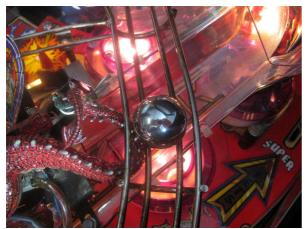
After some testings the ball is going through this. But if the ball stacks during gameplay you can remove the "pins" comming out of the tail with the help of a knife or a site cutter.
