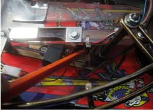
Put the flasher connector through this hole with the help of e.g. a pencil.
