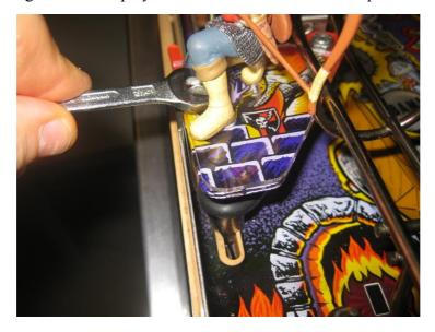
Left one, under the playfield (if there is no light up, switch the colors of the alligators) Left site of the lamp is +, right site of the lamp is GND
