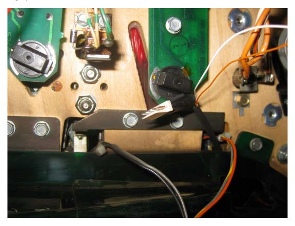
disconnect the original PCB Connector of the Magic Merlin Insert PCB (ignore the blue, green, red, black wire only in my pin for testing the merlin mods)
