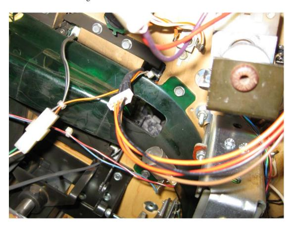
The flasher sandwitch cable is connected to the right down flasher
