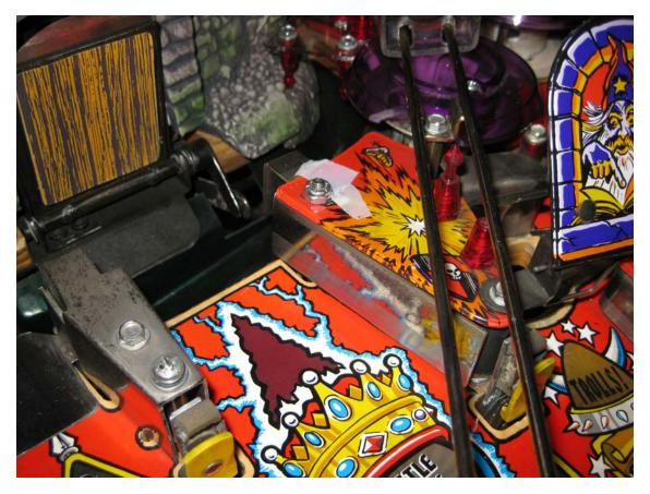
take care of the small colored wires when setting down the merlin (use the space we make for it under the merlin)
