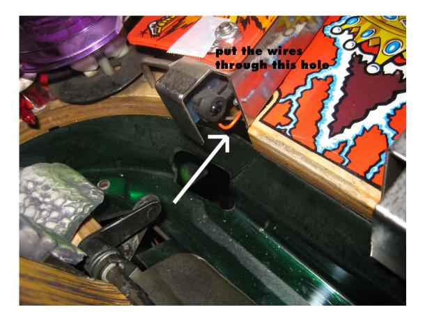
Insert first the flasher connector through the hole
